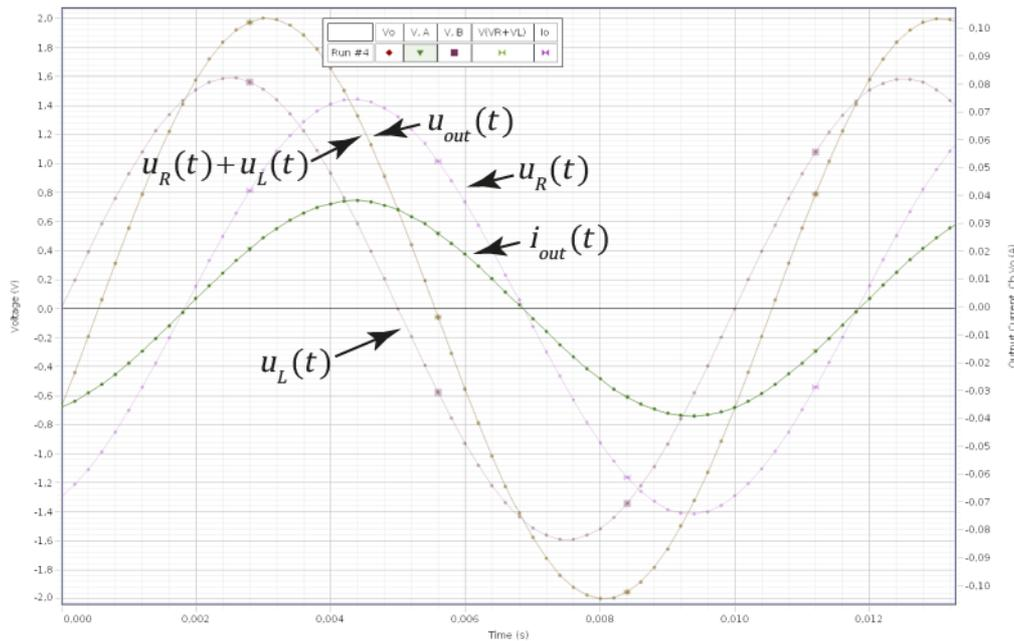
Fig. 4. Measured curves from a student lab-report for the task in Fig. 3. A tool in the software was used to calculate  $u_R(t) + u_L(t)$ . As can be seen in the figure this sum is identical with  $u_{out}(t)$ .
