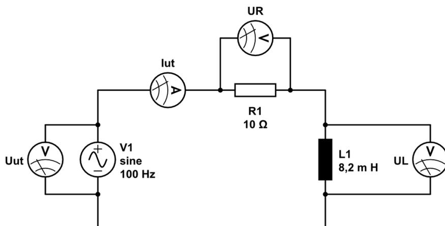
Fig. 3. An experiment in the first lab to investigate the validity of Kirchoff's voltage law. The output voltage  $u_{out}(t)$ , current  $i_{out}(t)$ , the resistor voltage  $u_R(t)$ , and the inductor voltage  $u_L(t)$  is measured by the interface and the results displayed on the computer screen (see Fig. 4). The interface generates a sinusoidal output voltage  $u_{out}(t)$  with a frequency of 100 Hz and amplitude of 2 V.
