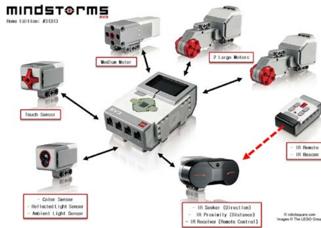
Fig. 2. Lego Mindstorms Sensors and actuators
