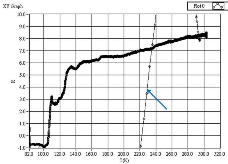
Fig. 4. Phase transition curves for temperature ascending (thick) and failed descending processes (blue arrow).
