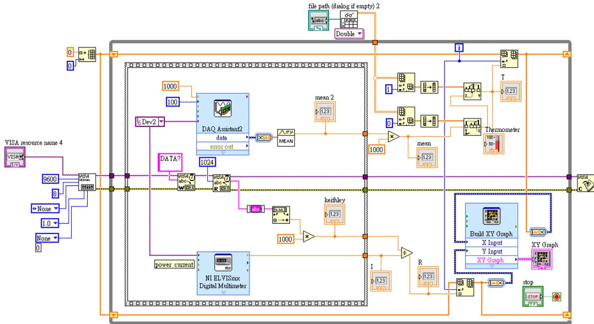
Fig. 2. Program of human-computer interface and data acquisition and analysis.
