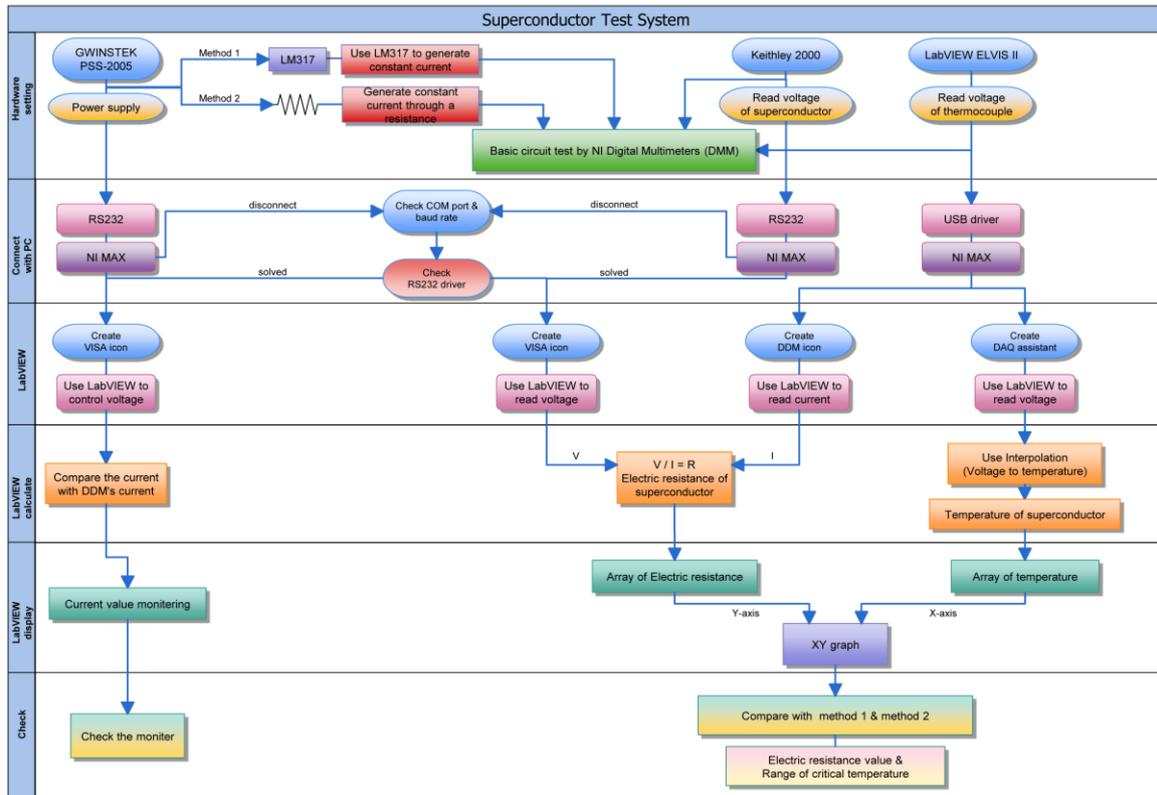
Fig. 1. A schematic diagram of the superconductor test system.
