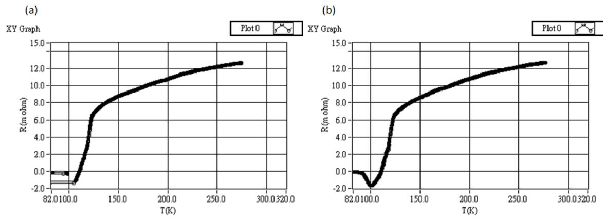
Fig. 3. Phase transition curves for (a) the GKE kit and (b) the LKE kit.
