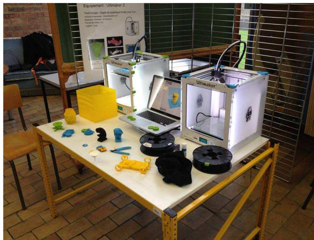
Figure 6: Ultimaker 3D printers of FabLab (University of Mons)
